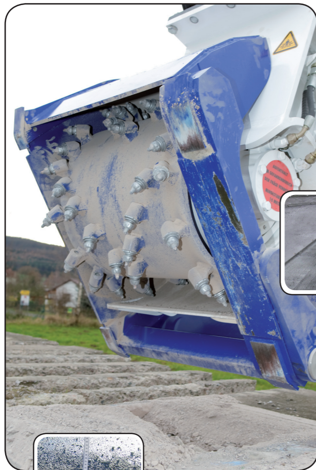
View from below of the cutter drum as used for planing concrete.
