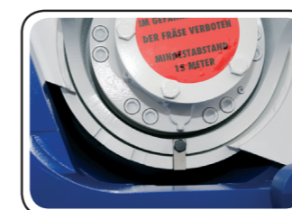
housing locking mechanism
