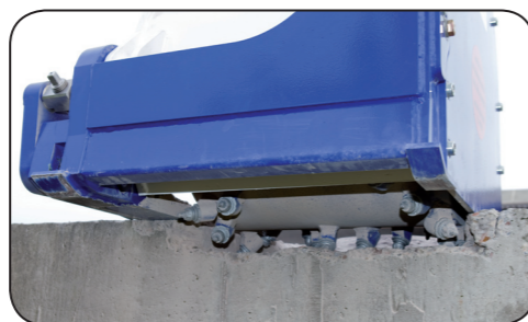
View from the front of the cutter drum as used for planing concrete.
