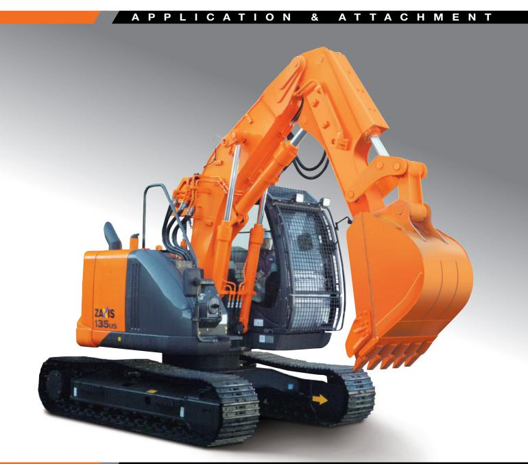
Model Code Engine Rated Power Operating Weight ZX135US-5B 73.4 kW (98 HP) 17 400 - 17 900 kg
